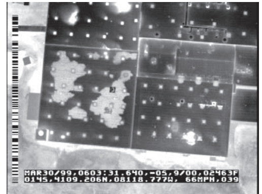
Aerial Infrared Roof Moisture Surveys
